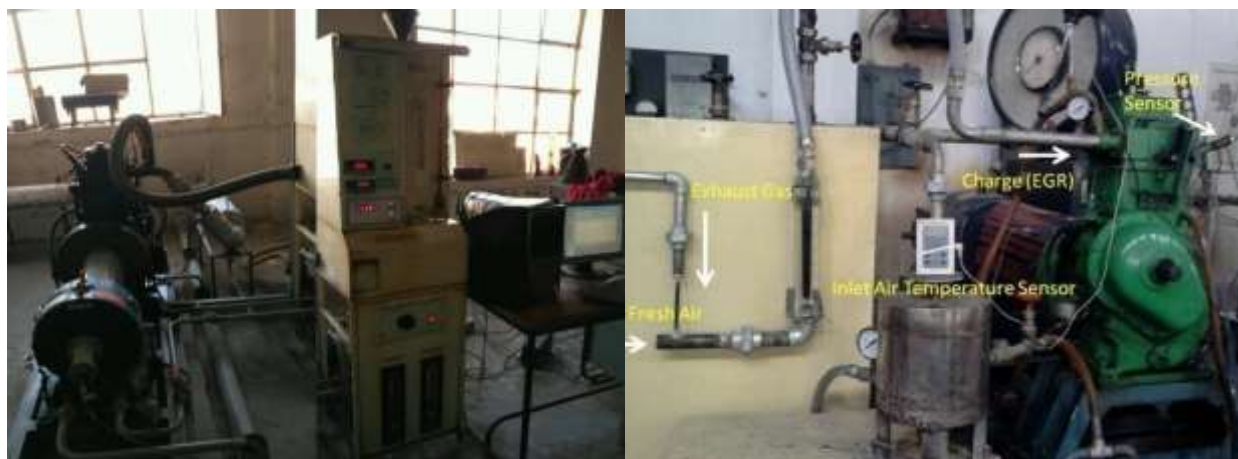
Figure 3.5: CI Engine used for Performance Analysis Figure 3.6: Photographic view of experimental setup showing EGR path
