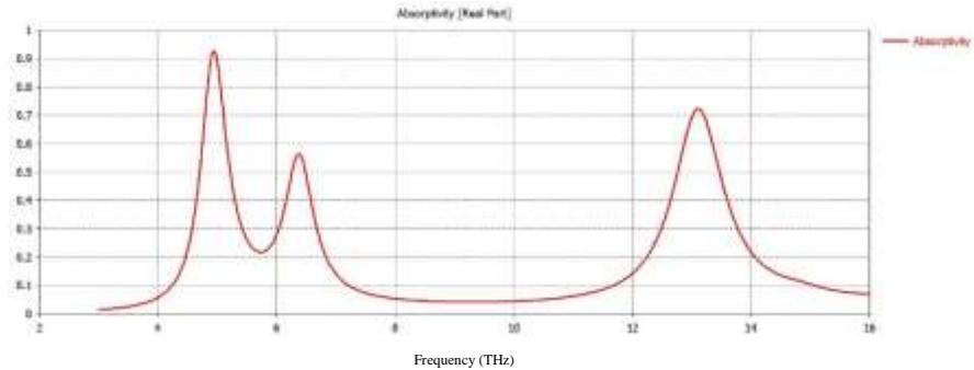
The absorption curve of structure-6 shows three significant peaks at 4.9, 6.3 and 13.2 THz resonant frequencies. The third absorption peak is improved when compared with the previous absorber structure. The introduction of semi circular graphite discs inside the square notch helped in achieving 3 significant absorption peaks with 92% being the highest.
