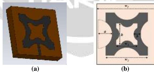
**Fig 1: (a) 3D view of the absorber, (b) Parametric view**
