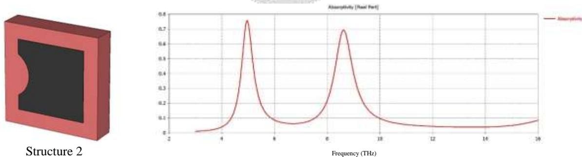
The absorption curve of structure-2 shows two significant peaks at 5, 8.7 THz resonant frequencies. The highest absorption peak is 75% at 5 THz frequency which is far better than the previous absorption peak in structure 1. This is because of the introduction of semi circular notch in one side of the graphite sheet.
