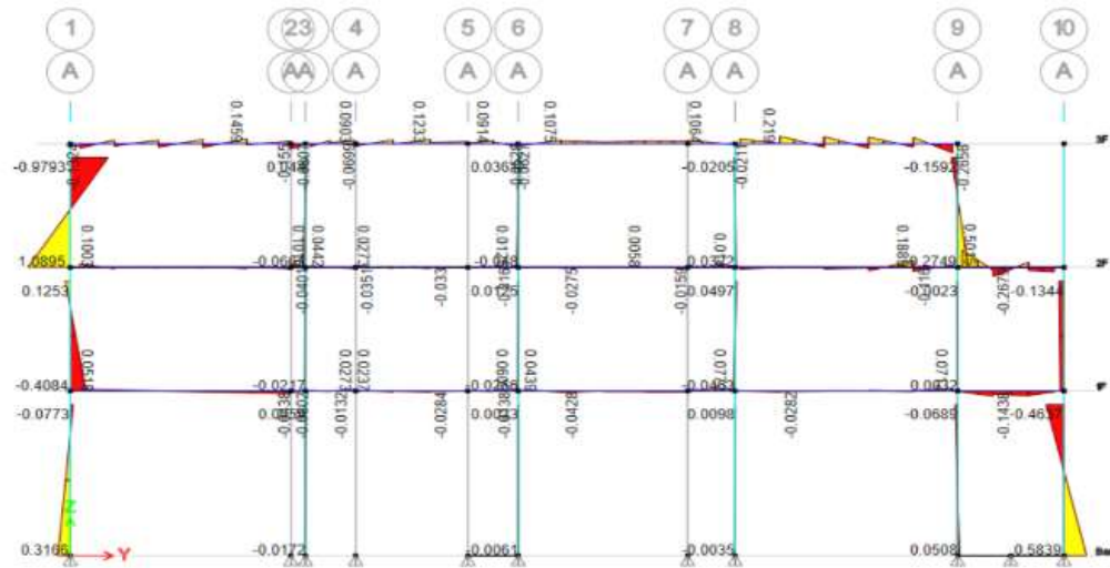
Fig.11: Analysis Using Etabs – L Shaped Column
