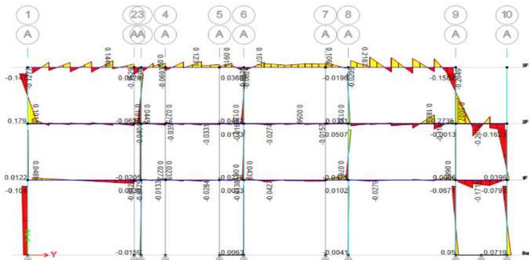
Fig.10: Analysis Using Etabs – Normal Column
