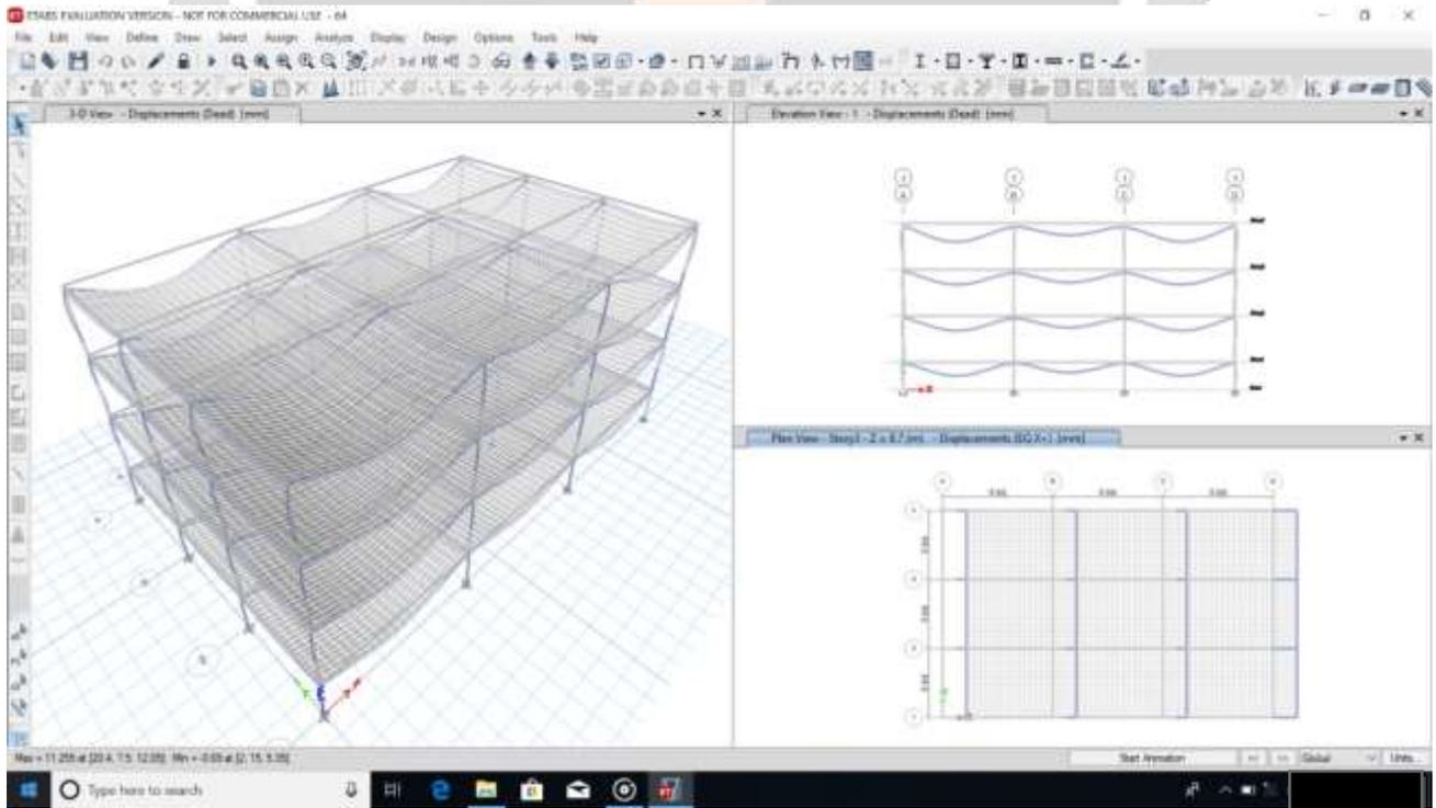
Fig -5: Deflected Shape of Structure
