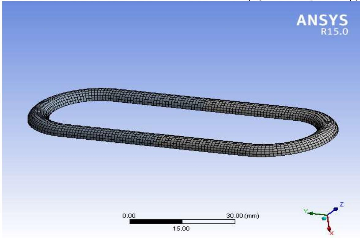
**Figure 3.2** Meshed domain of heat pipe.
