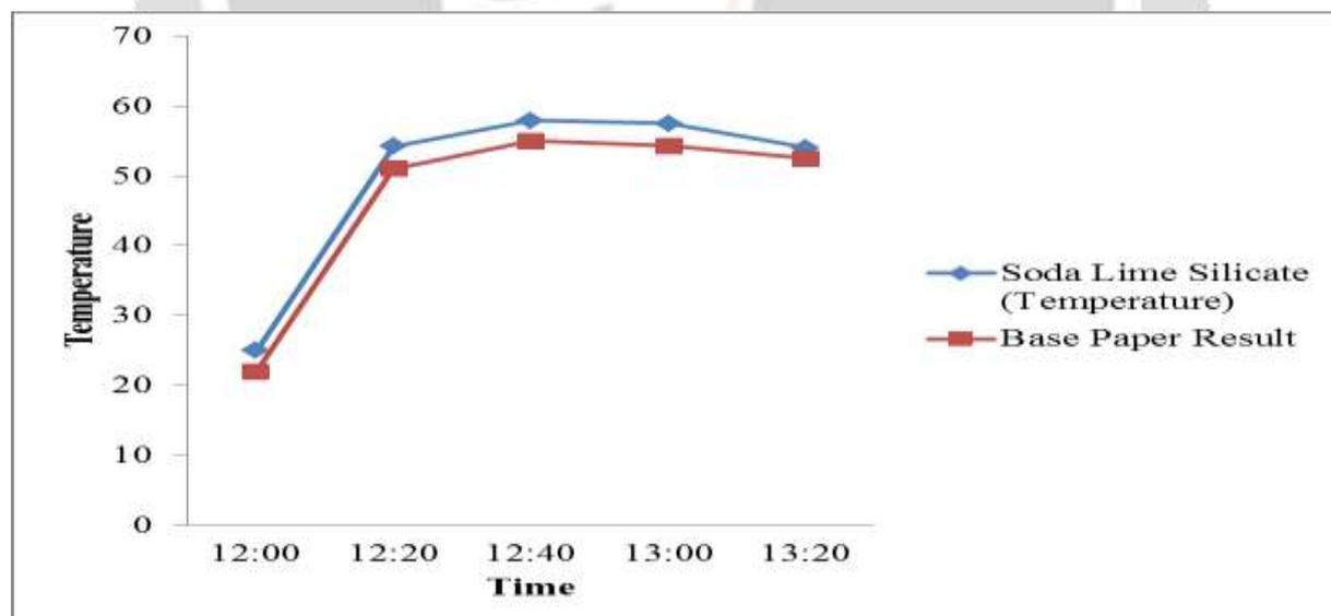
Figure 4.1 Temperature variation of Soda lime silicate glass evacuated tube on time.
