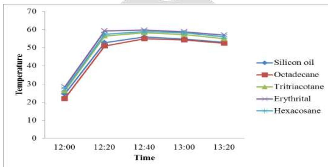
**Figure 4.8** Overall comparison of variation in Temperature for different nanofluid with the heat pipe with respect to Time.
