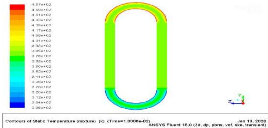
Figure 4.5: Temperature variations of heat pipe on 12:40.
