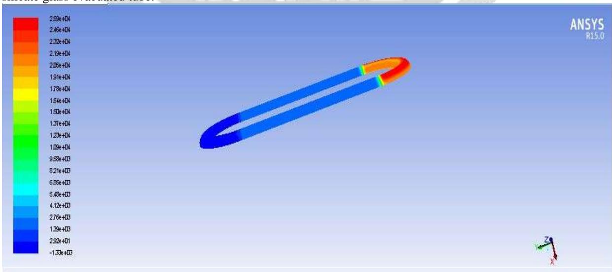
Figure.4.11 Temperature variation of heat pipe on 12:20.
