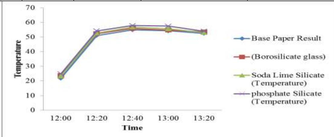
Figure 4.12 Variation in temperature on heat pipe wr.t. time
