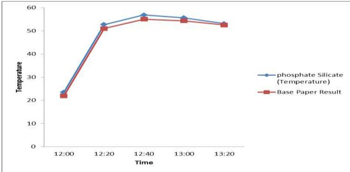
Figure 4.9 Temperature variation of phosphate silicate glass evacuated tube on time.
