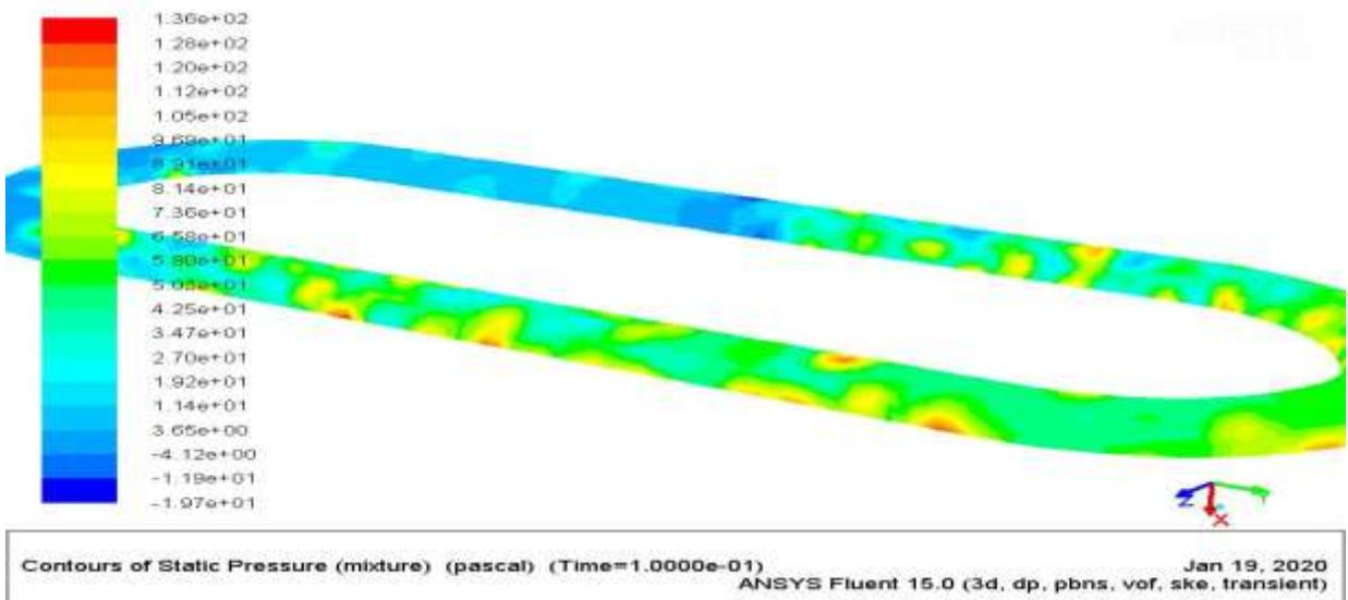
Figure 4.3: pressure variation of heat pipe on 12:00..
