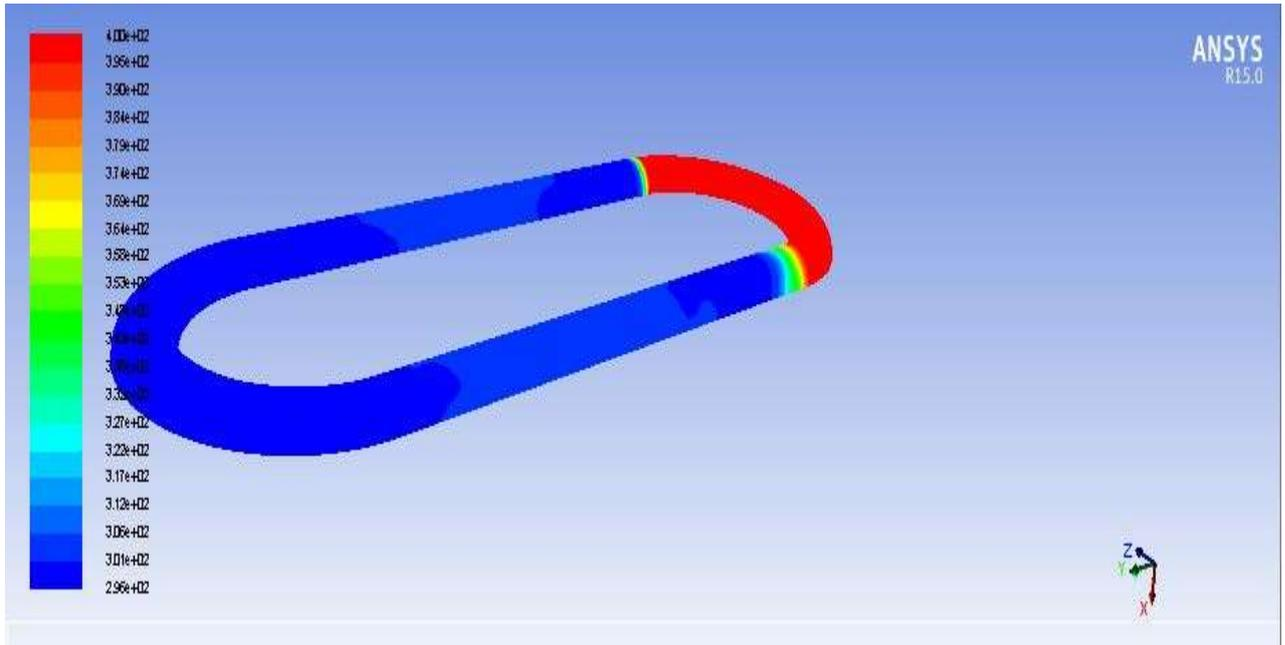
Figure 4.2: Temperature variation of heat pipe on 12:00.
