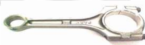
Fig.2 Connecting rod with nut and bolt
