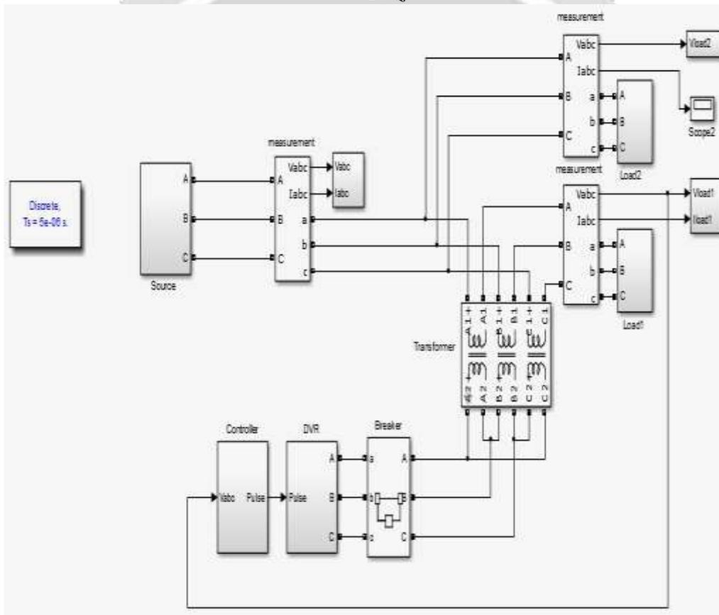
**Fig -1** Simulation model of the DVR system
