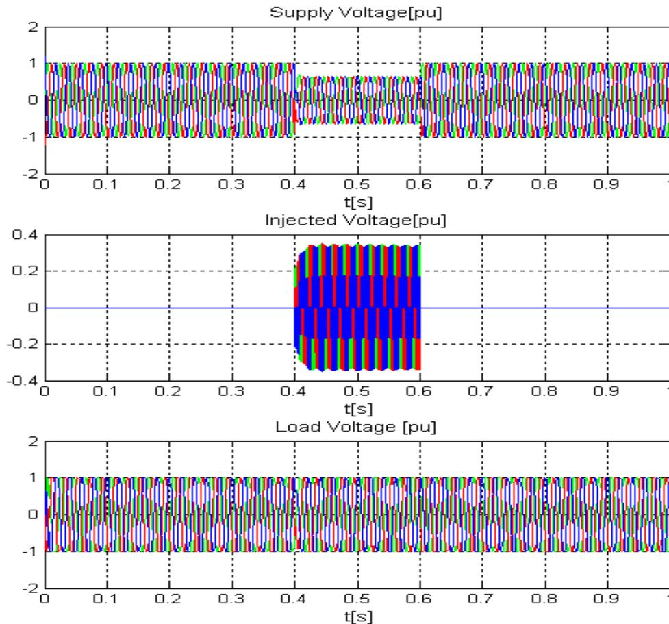
**Fig -2** Voltage, current of the supply source, load when using the DVR system during a three-phase voltage sag
