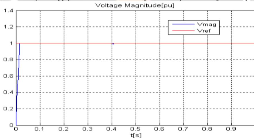
**Fig -3** Load voltage magnitude when using the DVR system during a three-phase voltage sag
