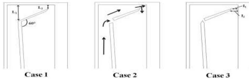
Figure 6.10: Top view of three different cases of impingement cooling of smooth channel.
