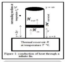
$t''(y) - \frac{\sigma P}{\mathcal{K} \mathcal{A}} [t(y) - t_s] = 0$  ......(1), where we assumed that the one end of the fin is connected to a heat source at y = 0 and the other end at y = infinity is free for losing heat into the surroundings. The source of heat is maintained at fixed temperature 'T' and  $t_s$  is the temperature of the surroundings of the infinite fin and is kept constant.
