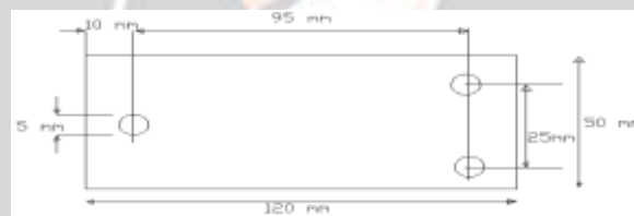
Fig-2 Dimensions of the sample leakage current test material
