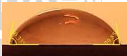
Fig-9 Surface contact angle of the insulator test material
