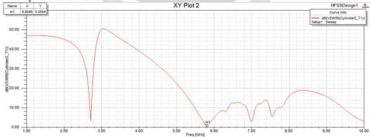
Figure 4.6: Graph of VSWR for f_0 = 5.8\text{GHz} .
