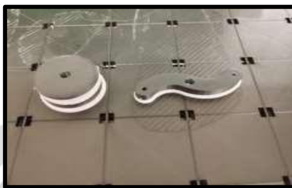
Fig-9: Final 3D printed of S-lever and Pulley Design
