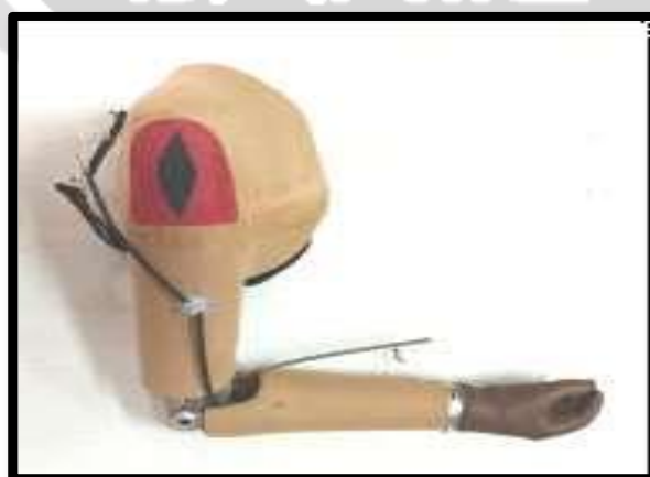
Fig-10: Newly designed excursion amplifier with SD prosthesis
