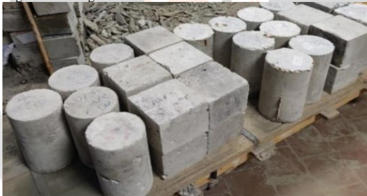
Fig. 2: Standard cubes and cylinders after casting.
