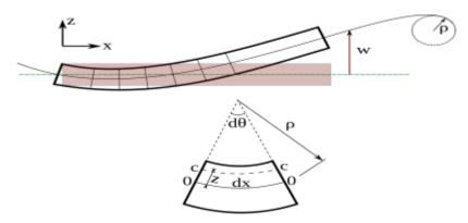
Because of the fundamental importance of the bending moment equation in engineering, we will provide a short derivation. We change to polar coordinates. The length of the neutral axis in the figure is  $\rho d\theta$ . The length of a fiber with a radial distance z below the neutral axis is  $(\rho+z)d\theta$  Therefore, the strain of this fiber is  $\rho/z$ .
