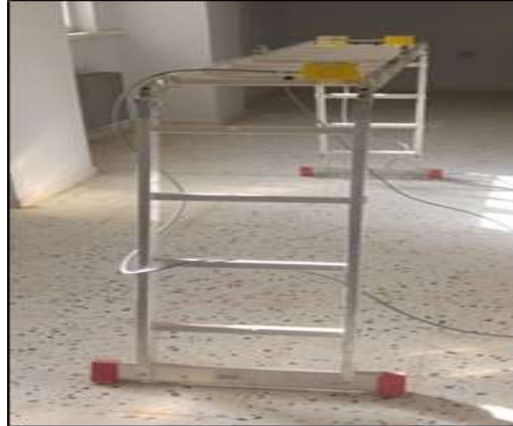
Fig -2: View of bench-scale aluminum bridge
