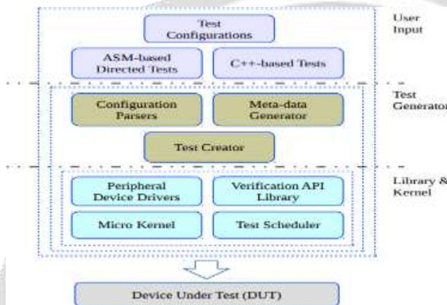
Fig: Different components of the software stack of STING
