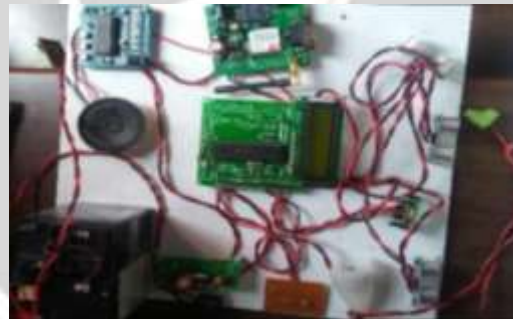
Fig -8: PIC16F877A MICROCONTROLLER BASED ANIMAL IDENTIFIER
