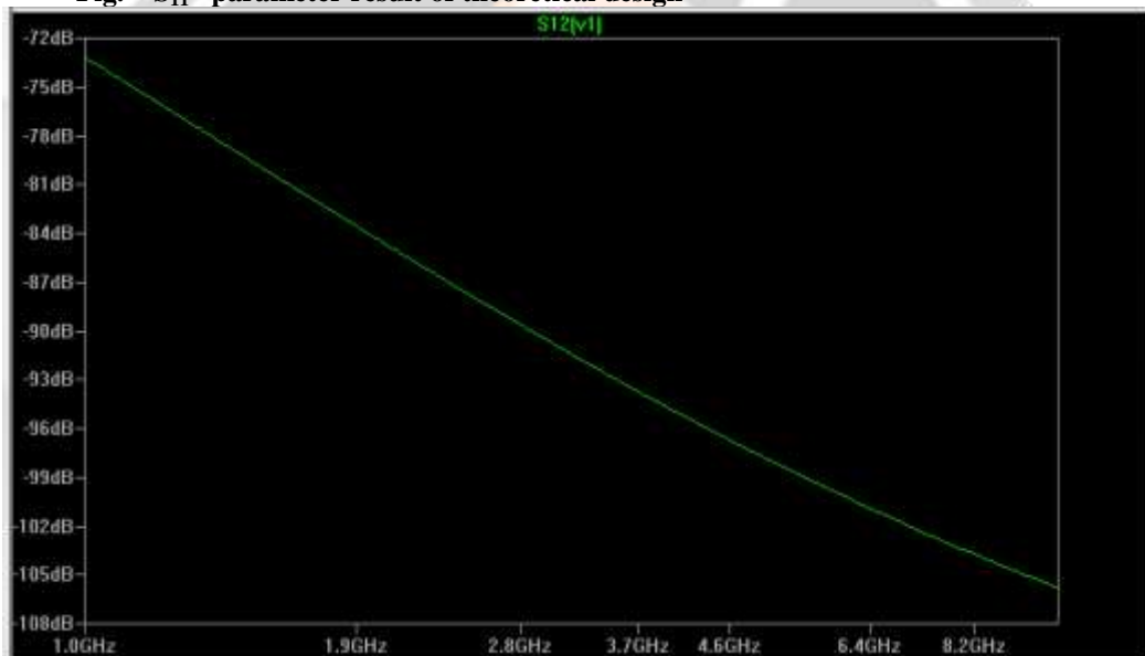
Fig. S 12 –parameter result of theoretical design
