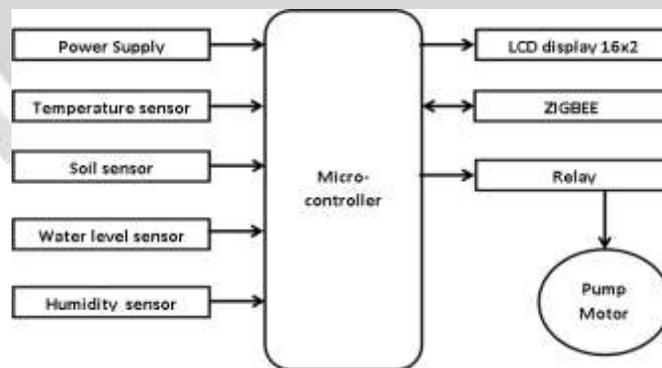
Fig2. Wireless Sensor Unit
