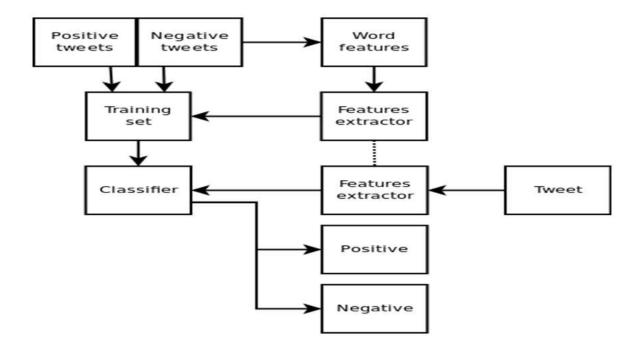
Fig2.Architecture Diagram of BTweet
