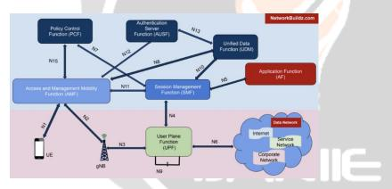
How it operates: Using the 5G New Radio Access Network, User Equipment (UE) such as 5G smartphones or cellular phones can connect to the 5G core and ultimately to Data Networks (DN) such as the Internet. The Access and Mobility Management Function (AMF) acts as a single-entry point for the UE connection, selecting the appropriate Session Management Function (SMF) to handle the user session based on the service that the UE has requested.
