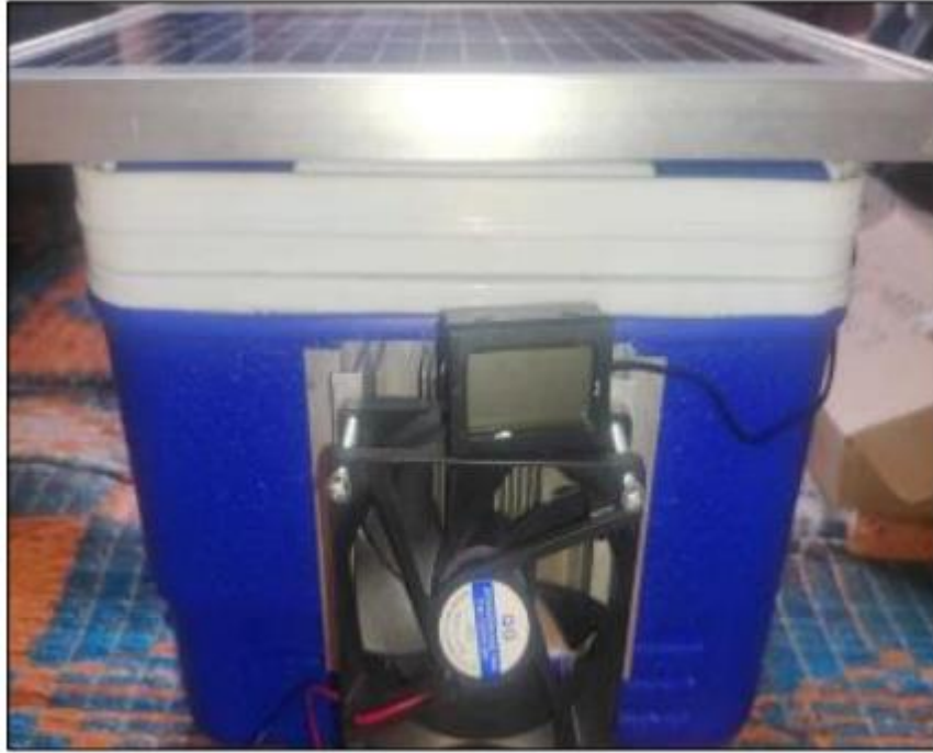
Figure 3 Fabricated model of the mini refrigerator
