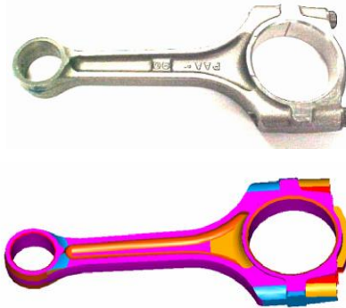
Fig- 2: The actual and the digitized connecting rods
