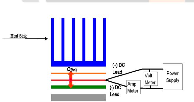
Fig 4.2 Schematic of the Testbed Layout
