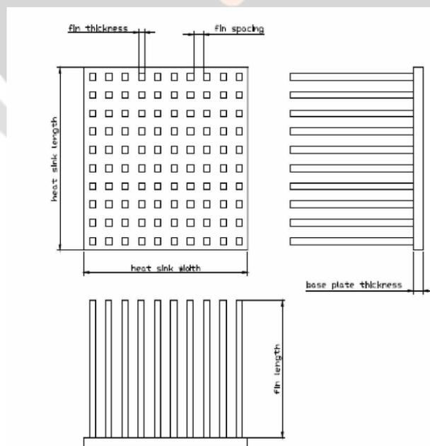
Fig 4.1 Heat Sink Design Parameters
