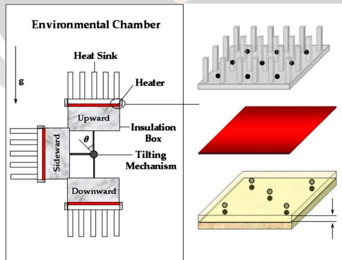
Fig.5.1 Schematic of the Experimental Setup with Different Orientation
