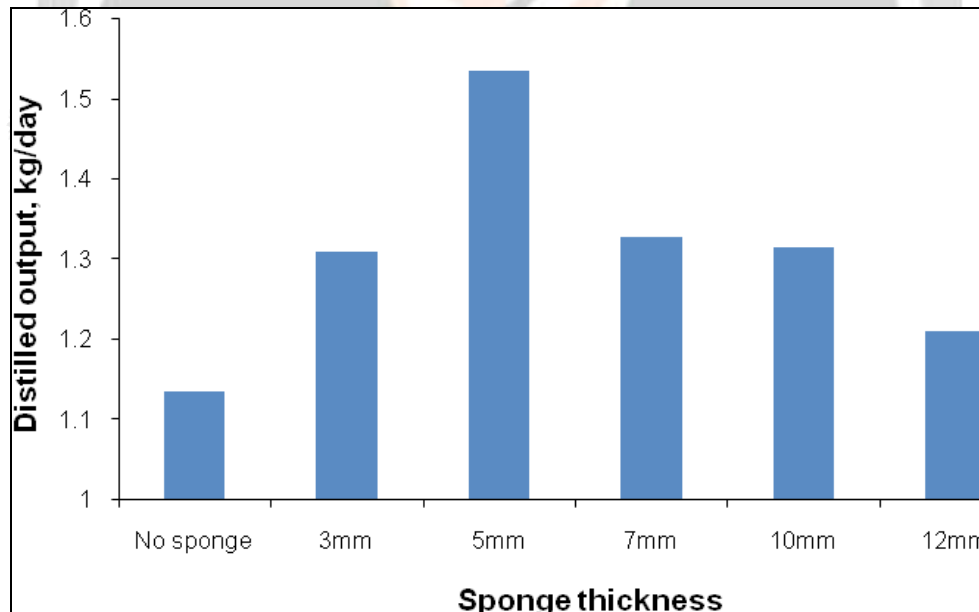
Fig. 9: Deviation in daily productivity with respect to various thickness of sponge liner [11]
