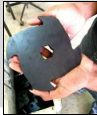
Fig. 4: Four blade cutter [8]
