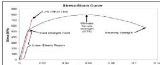
Fig.: Stress Strain Curve of Ductile Material
