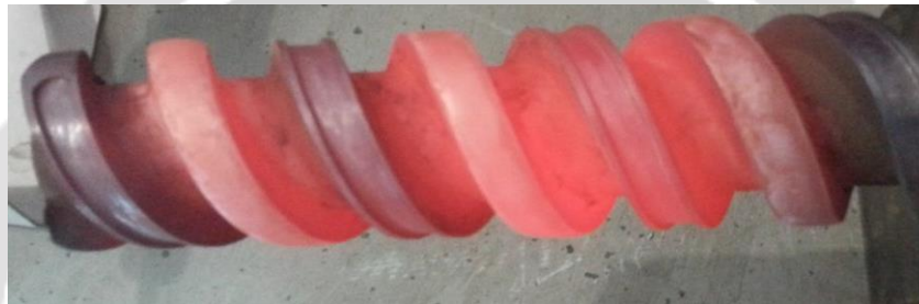
Fig – 2: Coating on extruder screw.
