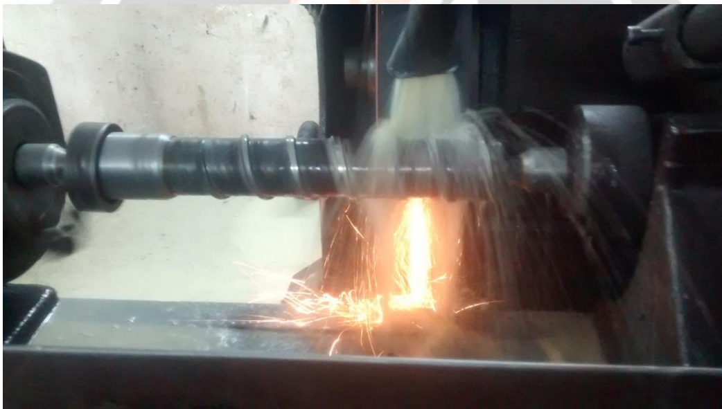
Figure 3 : Grinding on thermally sprayed workpiece
