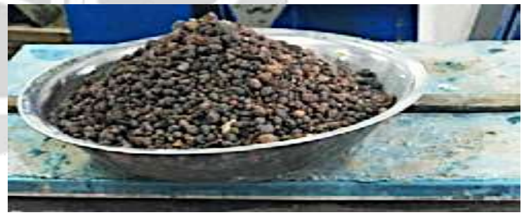
Figure. (15): fine grained expanded (zoom 3000%) clay aggregate
