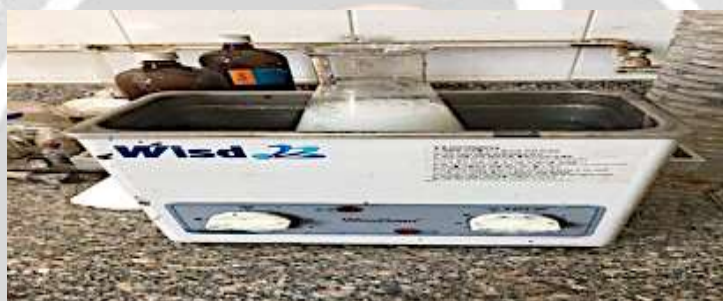
Figure. (28): Nano-silica solution making by ultra-sonication device
