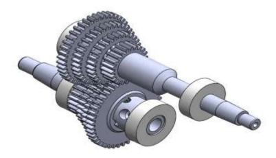
Fig. Cad model of gear box
