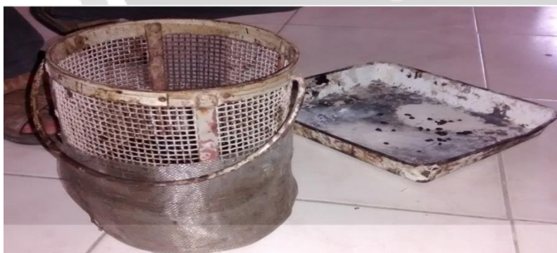
Fig 3.6: Wire Basket Assembly for Drain down Test
