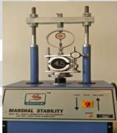
Fig-3 Marsha11 stability Test apparatus
