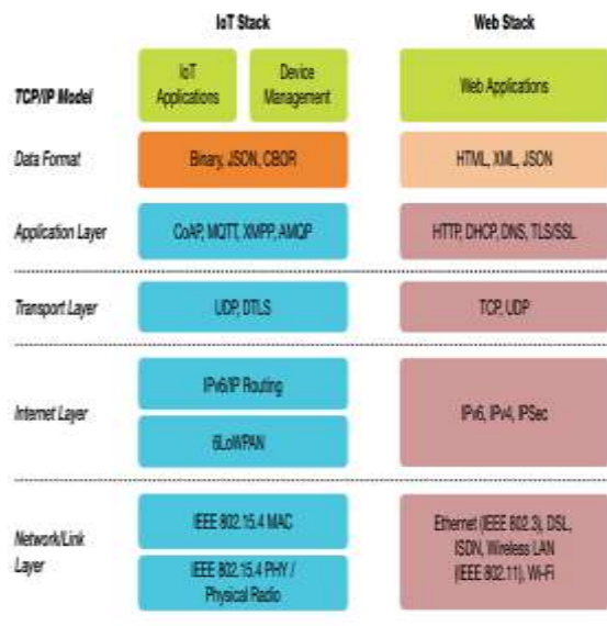
Figure 2. IOT PROTOCOL STACK
