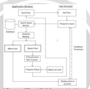
Fig. 1. Block Diagram of Filtered Wall Conceptual Architecture.
