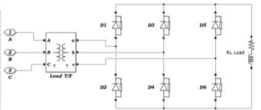
**Fig-7:** Non-linear load connected at the output section of the proposed system.
