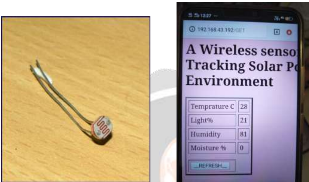
Fig.7 Light dependent resistor (LDR) with result
