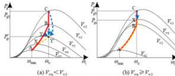
Fig. 5. Power characteristics of DFIG under active voltage control
