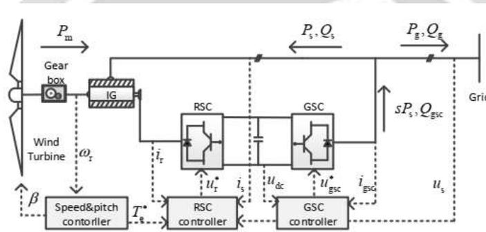
**Fig.2.** Schematic diagram of DFIG
