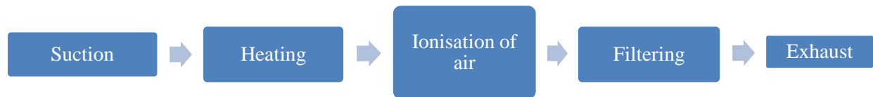
Fig1.1 Block diagram of various processes in smog cleaner.
