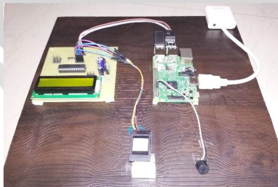
Fig -4: Hardware Model (with fingerprint Scanner)
