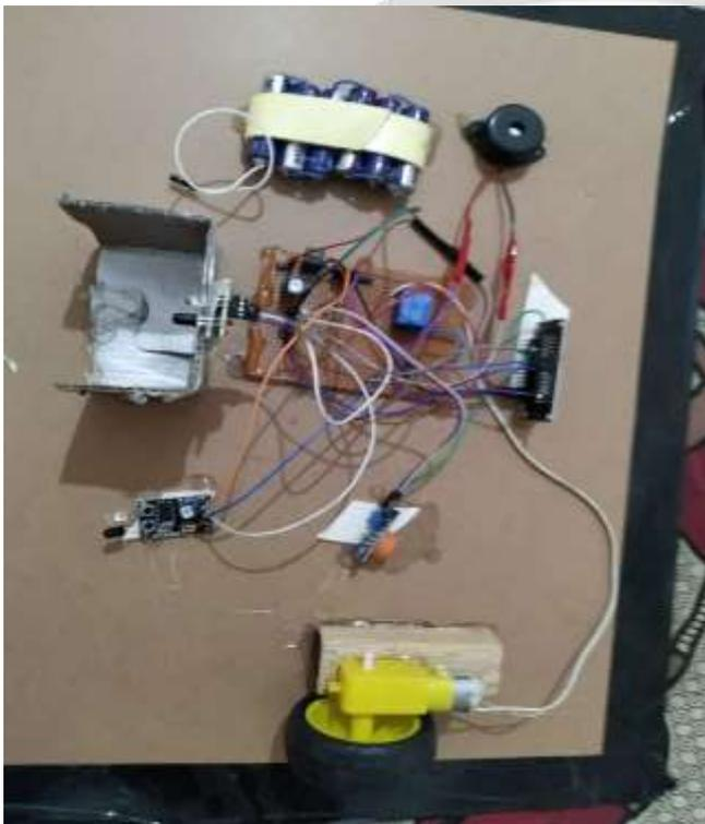
**Fig.2. Accident prevention breaking system by eye blink and alcohol detector.**
