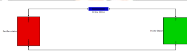
Figure 4.1: MATLAB simulation model for hvdc line power system includes rectifier station subsystem, inverter station subsystem and dc transmission line
