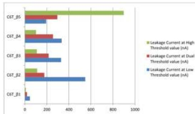
**Figure 5: 6T SRAM on various  $\beta$  ratios for write operation based on Leakage current**
