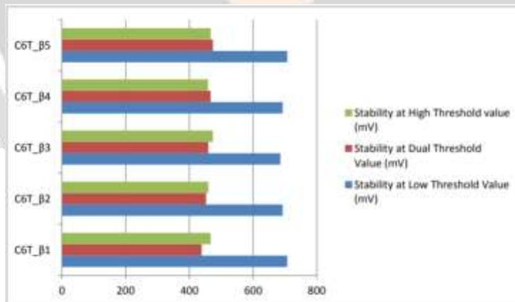
**Figure 3: 6T SRAM on various  $\beta$  ratios for write operation based on Stability**
