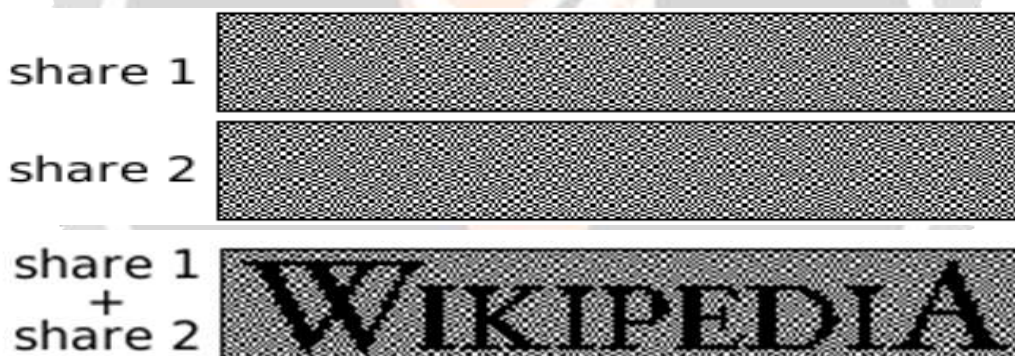
Figure 2. Visual cryptography example [15]
