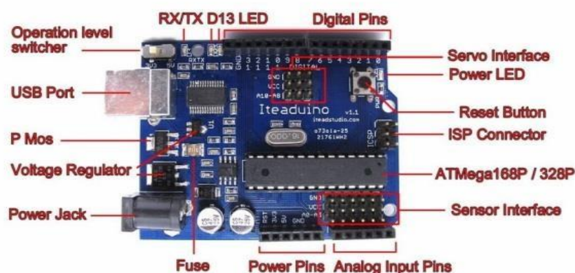
Fig2. Arduino Board Description
