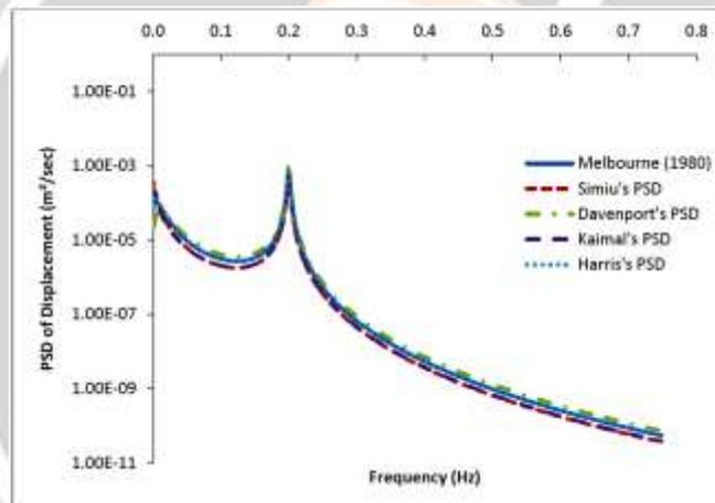
**Fig 5:** Response of CAARC building at  $U_h = 40\text{m/s}$
