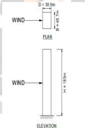
**Fig.2:** Geometric details of CAARC Standard Tall Building
