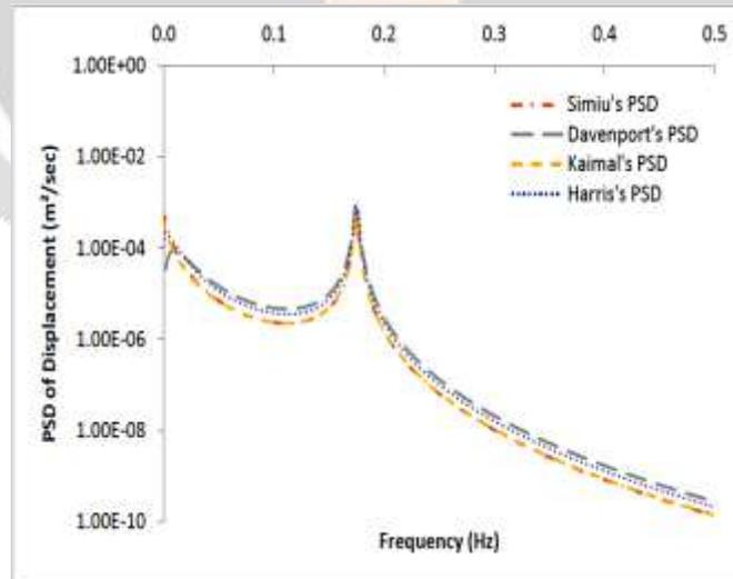
**Fig 4:** PSD of Displacement at height 200m
