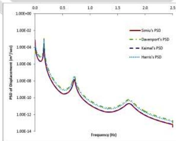
**Fig 7:** Response of 400m Chimney
