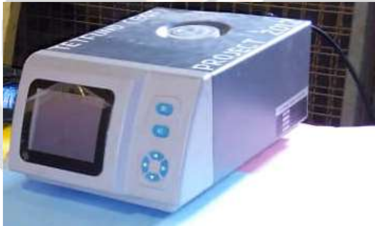
Plate II: SV-5Q Automobile Exhaust Gas Analyzer
