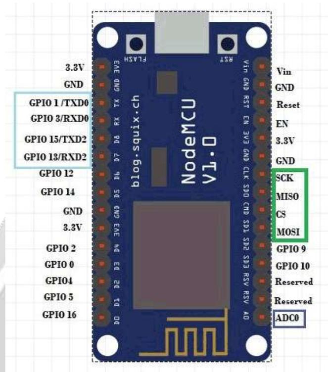
**Fig 2 : Pin Configurations of Node MCU ESP-12.**
