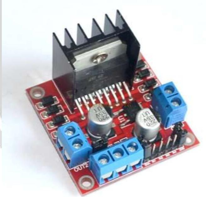
**FIG. 5: Motor driver controller L289N**
