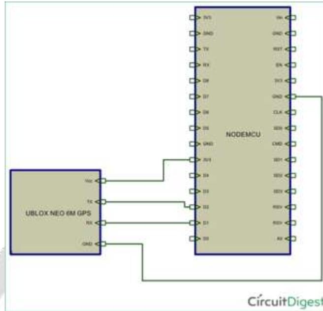
**Fig 4: Interfacing of GPS module Neo 6-M with Node MCU ESP-12 microcontroller**
