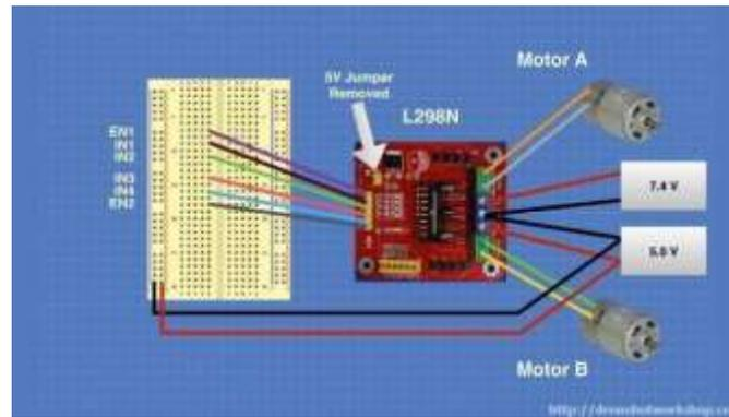
Fig 6: Interfacing of L289 motor driver controller with DC motors
