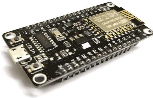
Fig 3: NODE MCU ESP -12
