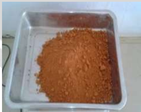
FIGURE 1. Crushed spent fire brick
