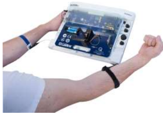
Figure 2. Myoelectric board to acquire SEMG
